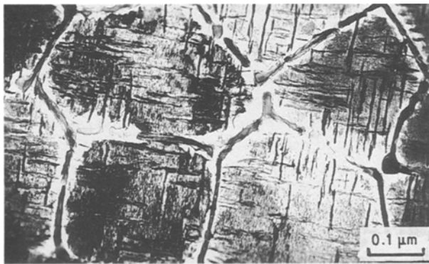
Figure 6 TEM micrograph of ribbon after ageing for 300 min at 700°C.
